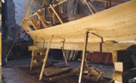
The second strake is fitted
