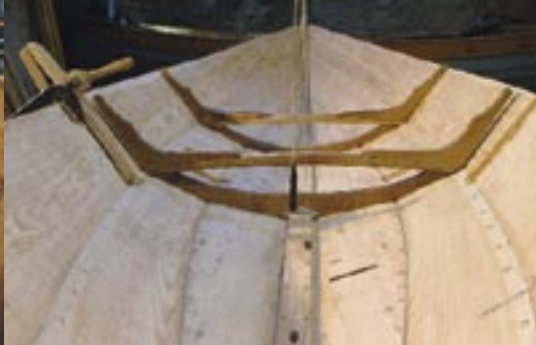
All planked up, frames fitted
