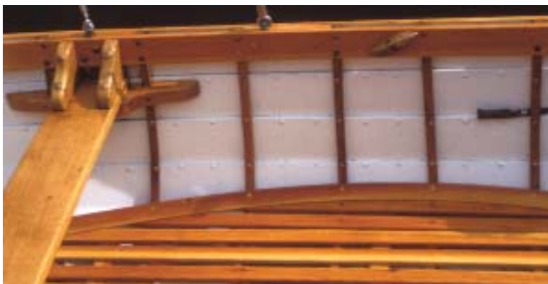
Top: Felicity John at Sail Caledonia 2003 when she won her first race. Above left: Steamed oak timbers at 9" (228mm) spacing. Above right: The bumkin allows the backstay to clear the boom.
